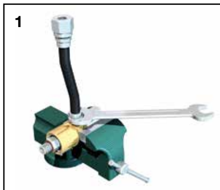
1 Mount housing in a bench vise and install hose.
